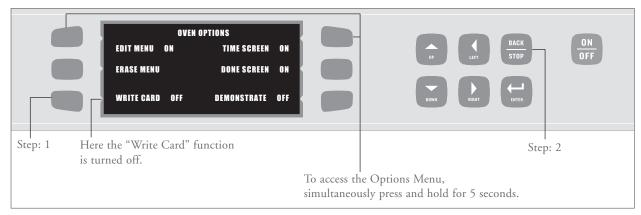
FIGURE 10: Enabling/Disabling the Write Card Function
